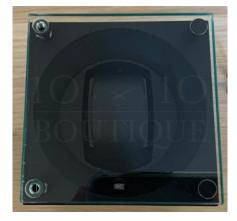
Sit the Acrylic Window (A) on top of the hinges with the countersunk holes facing upwards.Now place the Small Washers (F) in the countersunk holes as per picture right, and then insert the Window Screws (H) but only a couple of turns, DO NOT tighten yet.
